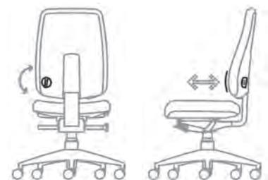
This maintains the S-shape of the backbone and encourages an upright sitting posture. Optional: customizable Schukra lumbar support adjustment. The maximum protrusion is achieved with just 1/4 turn.
